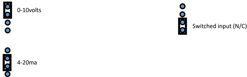
Once the jumpers have been set for each zone the dip switch must also be set. Use the first bank of 4 switches. The switch for each zone chooses between 4-20ma (on / up) or 0-10v / switched input (off / down)
